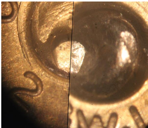
Figure 3: Firing pin impression match on cartridge case.
