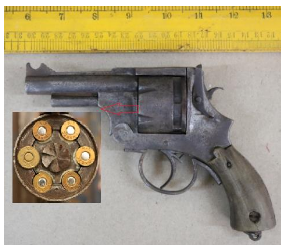
Figure 1: Improvised six chambered revolver.
