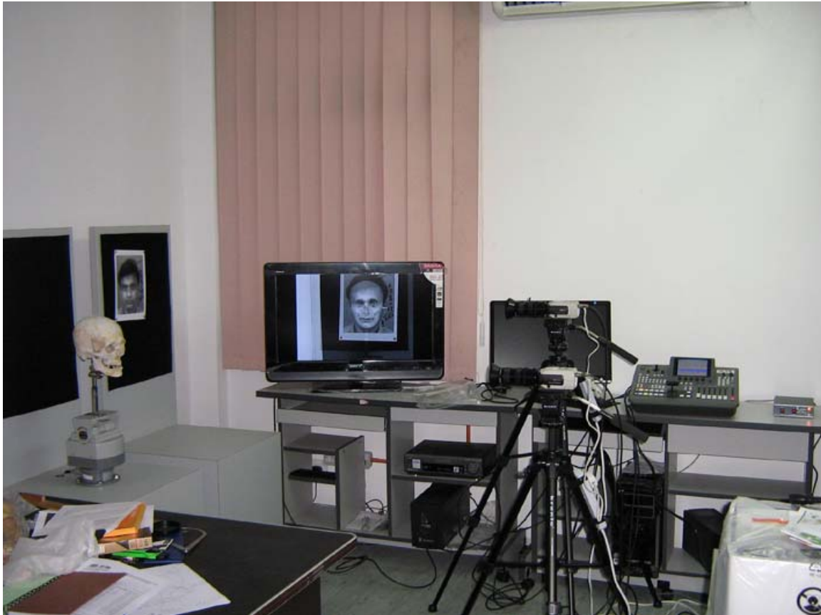
Fig. 1: Computer Aided Video Superimposition Device (CAVSID) fabricated in Universiti Sains Malaysia, the first of its kind in Malaysia.
