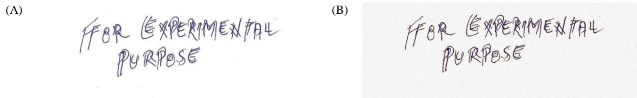
Figure 4: (A) The original control scanned document of blue ball point ink strokes; (B) No separation of the ink observed by change in color intensities of two same blue ball point ink strokes.
