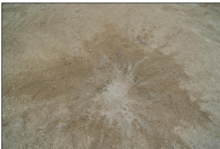
Fig 4: FO flash pattern formation the in the crater (60:40)
